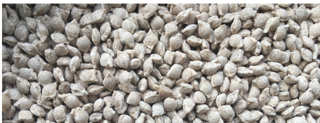
Figure 2. Fertilizer granules produced with the Granupaktor.
