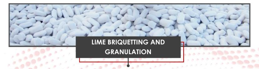
**EURAGGLO** offers a briquetting, compaction and granulation process based on the technology of roller compactors. This process allows the agglomeration of various dolomitic or high-calcium quicklime coming from screening at the end of the lime kilns.
